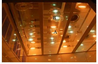
Figure 8. High Pressure Sodium (A) and Metal Halide (B) lamps in a growth chamber.
